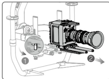
2. Unlock the lever on the adapter. Then, secure the camera on the tripod by sliding the camera into the adapter until the safety lock engages and the camera is balanced. Then, lock the lever to secure the camera in place.
