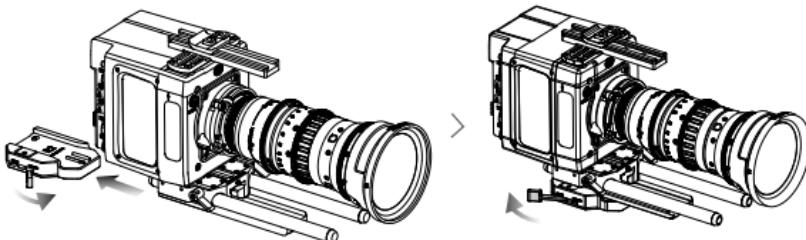
3. To remove the camera from the adapter, unlock the lever, and then slide the camera base plate out of the adapter while holding down the safety lock release (located on the side of the adapter).
