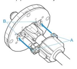
**3.** With leading edge of roll paper facing forward as shown, insert Roll Holder from right side of roll. Insert firmly until roll paper touches flange (A) of Roll Holder.
