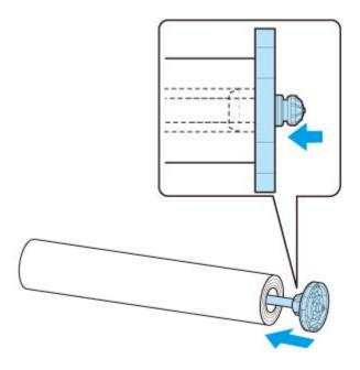
3. Load roll paper in printer or roll unit. (See "Loading the Upper Roll on the Printer.") (See "Loading the Lower Roll on the Roll Unit (Option).")
