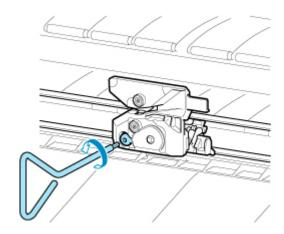
7. Remove cutter blade while holding D.
