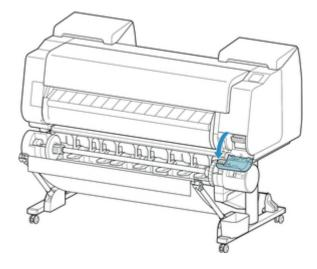
**6.** Hold the used maintenance cartridge by the grip (B) with one hand and put your other hand under the maintenance cartridge to hold it firmly on the bottom, keeping it level as you pull it out.
