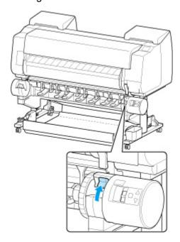
**3.** Hold flanges (A) so that roll holder's black gear is on left, align roll holder shaft with roll holder slot left and right guide grooves (B), and load.
