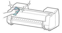
Open the top cover and output guide and clean parts that come in contact with paper (A, B), sensor (C) and window on the back side of the top cover.
