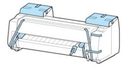
**3.** If using roll unit, refer to Setup Guide provided with roll unit and attach roll unit to Stand.
