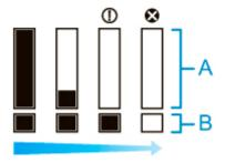
If the touch screen indicates to replace the ink tank, replace the ink tank. If a message is displayed indicating to check the remaining ink levels, or after tasks that consume a lot of ink such as large-format printing or head cleaning, check the remaining levels and replace ink tank as needed.
