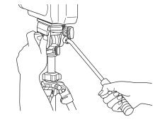
When loosening either the knobs, or the levers, take precaution by keeping a firm grip on the handle until the pan head is locked down.
