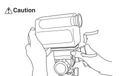
The video camera should be attached from the front of the quick release shoe.
