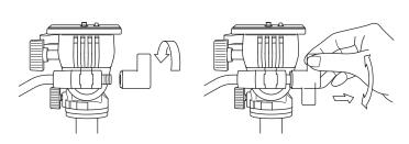
Please remove the handle lock knob and then, insert pan & tilt handle in the axis hole.
