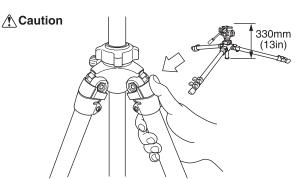
After choosing the desired leg angle, securely push in the adjustment lock. By using the optional short center column, you can obtain the lowest camera height of 330 mm (13").
