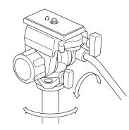
Loosen the panning lock knob, and the head will rotate along the horizontal direction.
