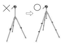
To avoid unnecessary camera vibrations, try to keep the center column height to a minimum.
