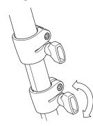
To extend, or shorten a leg, loosen the leg lock knob by turning it counter clockwise.
