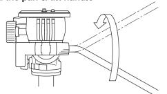
Pan & tilt handle can be changed to the left-hand if you reverse it. Please level the vertical tilt lock knob and then, insert pan & tilt handle from the front.
