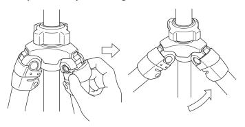
To change the angle of each leg, close the leg slightly, and then pull the leg angle adjustment lock out.
