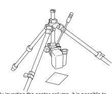
By inverting the center column, it is possible to do copy, and close up work. Follow the same procedures in order to replace with optional short center column.
