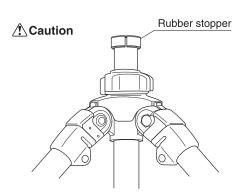
Make sure to re-attach the rubber stopper, in order to prevent the center column from falling
