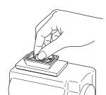
Please set the camera mounting screw and the retractable camera positioning pin to holes at the camera side.
