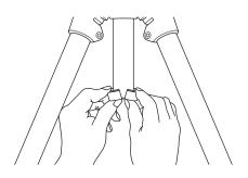
Remove the rubber stopper from the bottom of the column.
