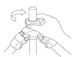
Insert the center column from the lower side of main body, and tighten the locking collar and the center column stopper.
