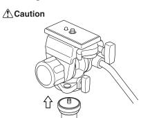
Always remove the pan head when replacing the center column.
