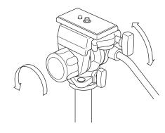
Loosen the tilting lock knob, and the head will tilt back and forth.
