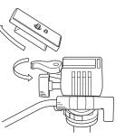
Remove the quick release shoe turning the lock lever.
