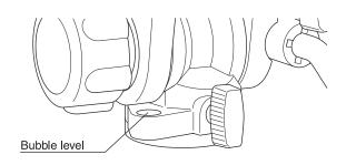
Bubble level is built-in for vertical and horizontal positioning.
