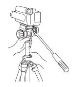
Hold onto the pan head with one hand, and loosen the center column stopper and the center column locking collar with the other hand.
